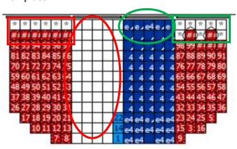
Floating crane needs full vessel hull to moor against while handling breakbulk, eg. handling breakbulk in first bays is impossible due to curve of vessel bow. Same is valid for aft side of vessel
